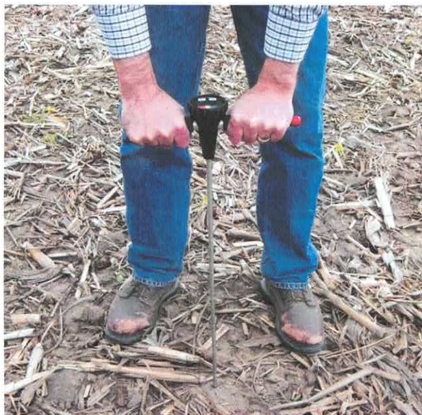
Picture 1: Using the Soil Compaction meter to determine soil compaction. Photo Credit: SpotOn.
