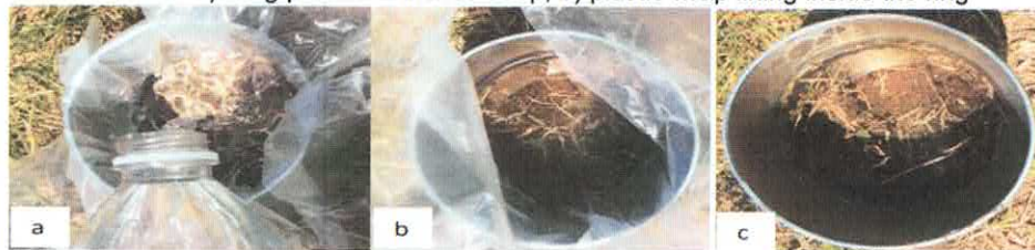
Picture 2. a) 1 inch of water, b) removing plastic wrap, c) water infiltrating the soil
